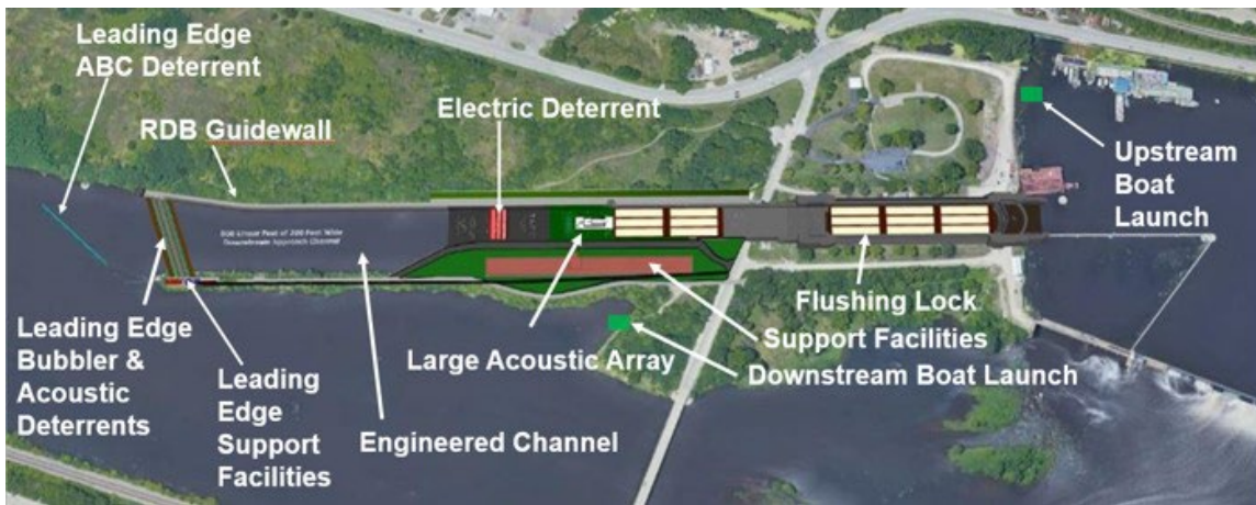
Figure 14 — Recommended Structural Plan – USACE Brandon Road
