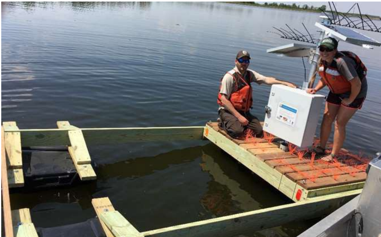
Figure 14. USFWS and USGS staff deploy a real-time telemetry receiver in the Intensive Management Zone of the UMR. Photo courtesy of USFWS.
