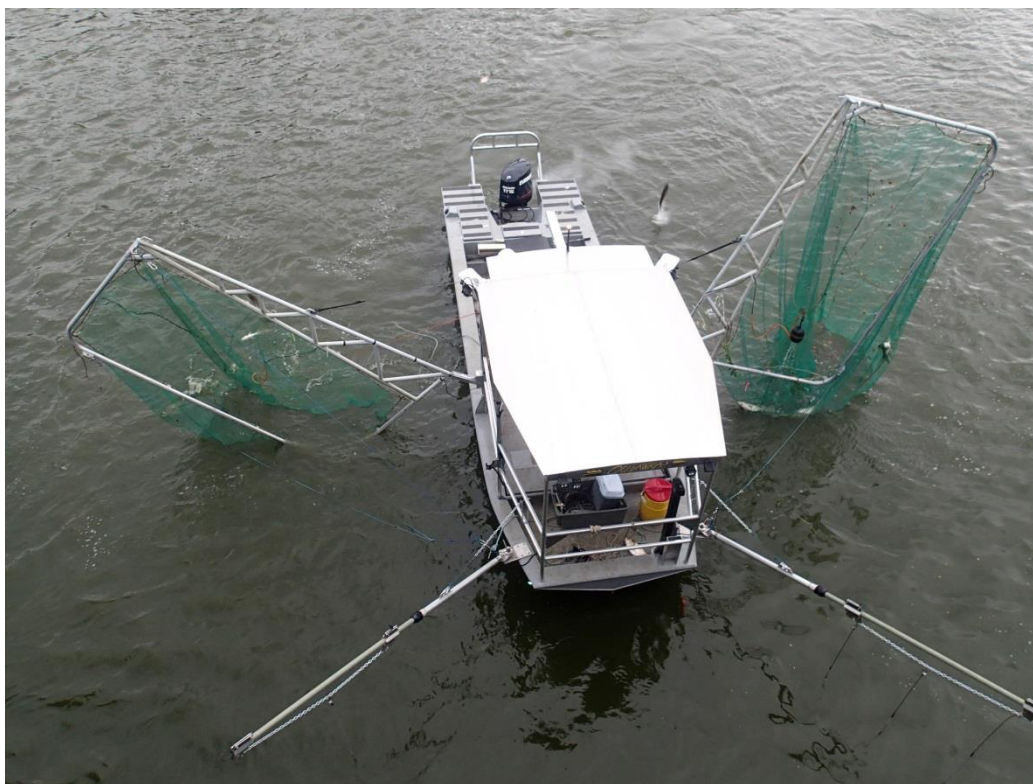
Figure 6. An aerial view of a paupier shows the rigid frames on both sides and booms extending in front of the boat.
