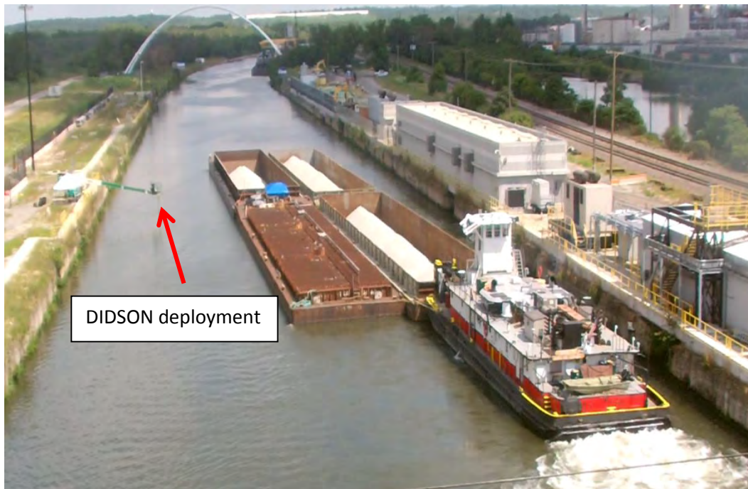
Figure 5. Northbound commercial barge tow traversing the Electric Dispersal Barrier while the DIDSON deployment continues to collect data.
