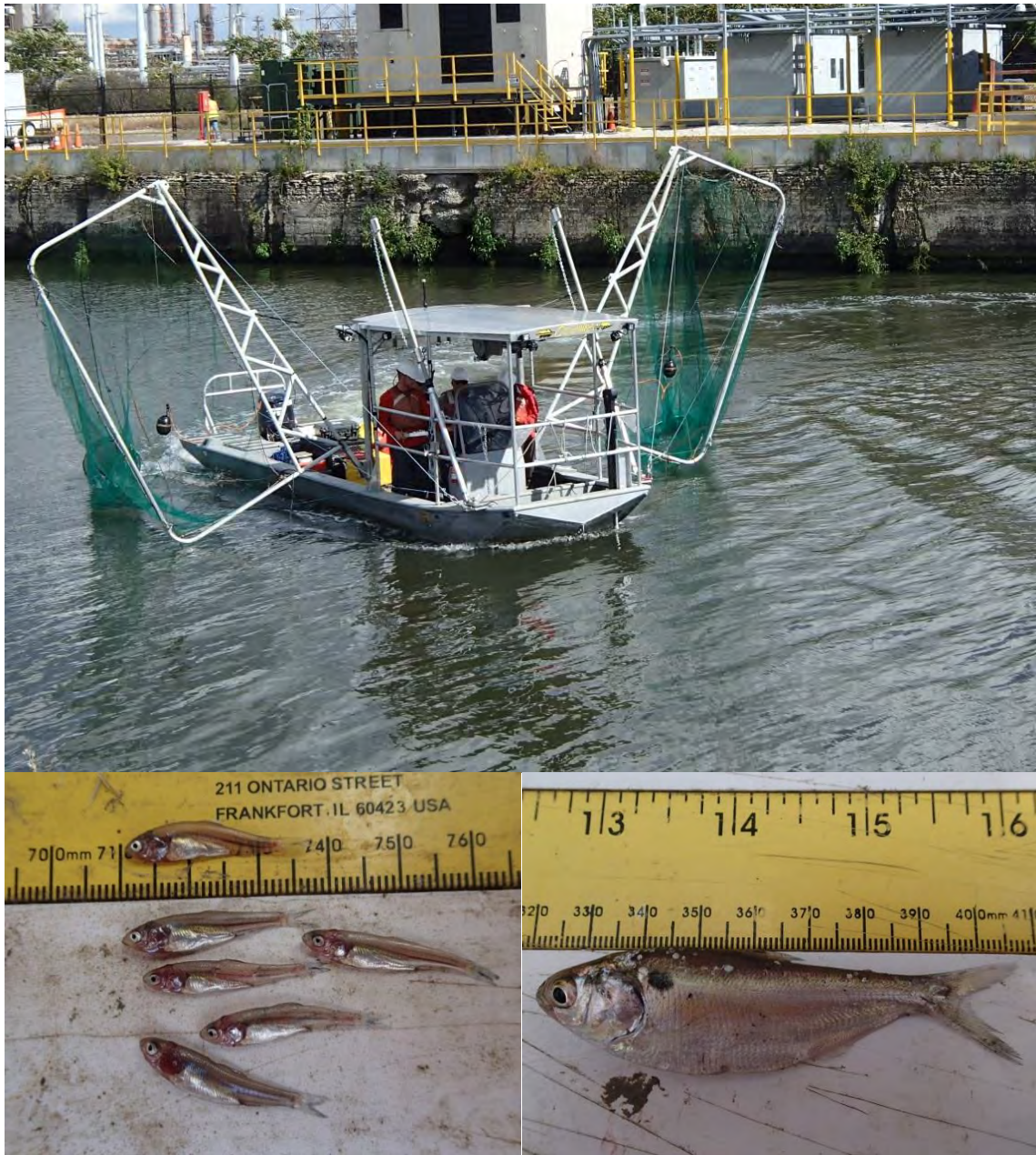
Figure 3. Paupier butterfly trawl net deployment used to capture fish within the vicinity of the CSSC Electric Dispersal Barriers. The nets extend over the sides of the vessel and are lowered and raised into and out of the water at precise locations. Juvenile Gizzard Shad captured over the Electric Dispersal Barrier system during July 2015.
