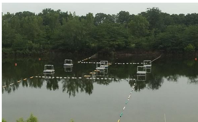
Field testing the use of complex sound to move Asian carp.
