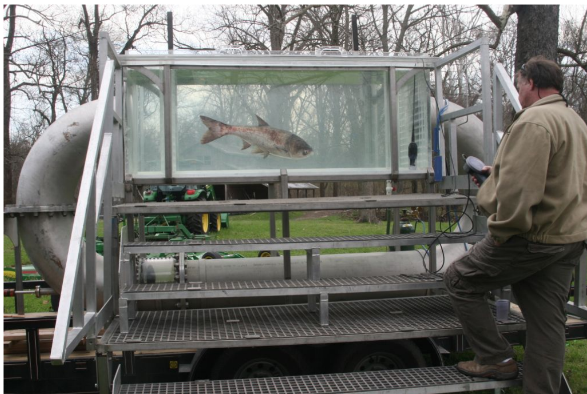
Figure 1: ERDC-EL researchers in trial testing a brand new and enlarged version of a Brett swim tunnel at a field location using the same water in which the fish was captured from. The swim tunnel is mobile and can be taken on site, which reduces handling and holding stress on the species of interest.
