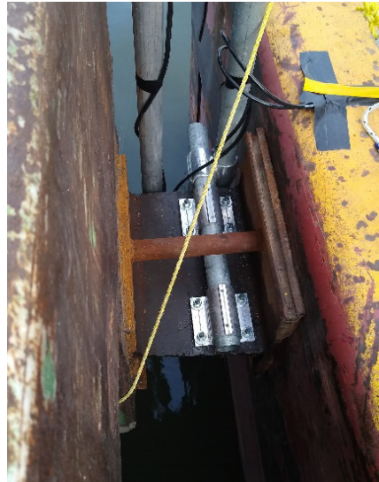
Figure 2. A photo of a 15-foot welded steel spacer designed to separate the rear-most and middle barges and allow for gear deployment in the junction gap. An ARIS 3000 Explorer multibeam sonar is also shown mounted to the spacer.
