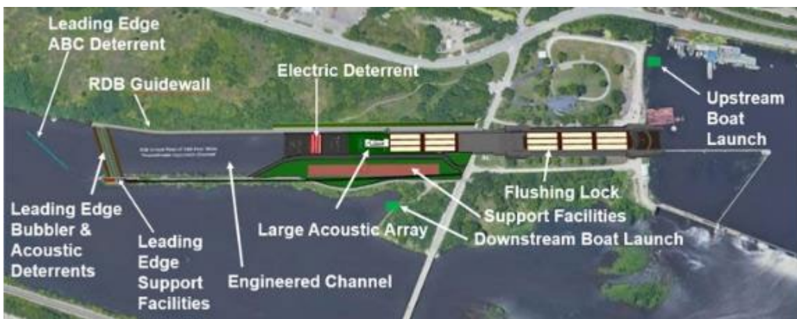
Figure 15. Recommended Structural Plan – USACE Brandon Road
