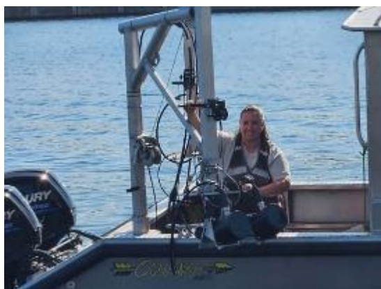
Figure 28 — Deploying Hydroacoustic Transducers
