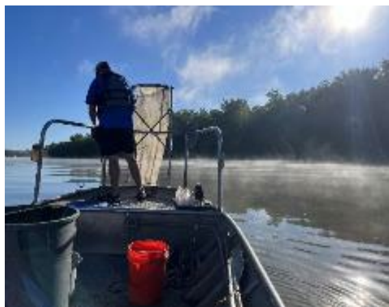
Figure 38 — Deploying an Ichthyoplankton Push Net
