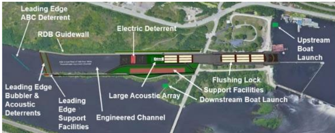
Figure 15 — Recommended Structural Plan – USACE Brandon Road
